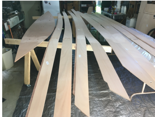
Photo 3: "Puzzle pieces" assembled into hull components.
