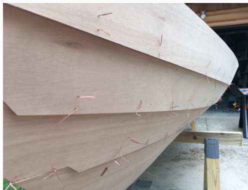
Photo 4: Closeup of the wire "stitches" that hold things together until the epoxy is applied.
